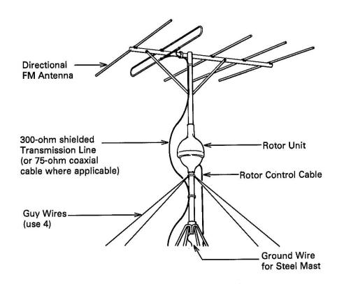
Another important factor is the type of lead-in wire to use. Unshielded lead-in wires, such as 300-ohm twin lead, can act as an omnidirectional antenna, and can cancel the directional benefits of your antenna. Therefore, we recommend using a balanced, shielded 300-ohm cable or a coaxial 75-ohm cable with a 300-to-75 ohm matching transformer at the antenna. These types of shielded cable effectively prevent the lead-in from contributing to multipath distortion.
