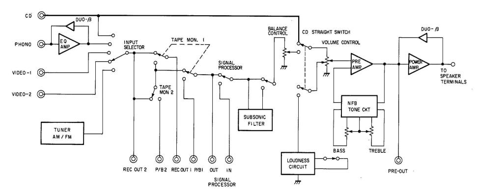
By bypassing these functions, the shortest direct path to the power amplifier is thus achieved, ensuring the best accuracy, imaging and impact.
